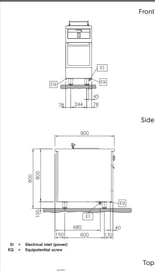
Electric Supply voltage: 400 V/3N ph/50/60 Hz Total Watts: 10 kW **Key Information:** Number of wells: Usable well dimensions (width): 240 mm Usable well dimensions 225 mm (height): Usable well dimensions 380 mm (depth): Well capacity: 12 lt MIN; 14 lt MAX Thermostat Range: 100 °C MIN; 180 °C MAX External dimensions, Width: 400 mm External dimensions, Depth: 900 mm External dimensions, Height: 800 mm Net weight: 75 kg On Base;One-Side Configuration: Operated Sustainability
